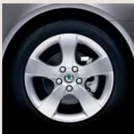
Pegasus alloy wheels 7.0J x 17" with 225/45 R17 tyres. Extra equipment for the Ambiente and Elegance versions.*
