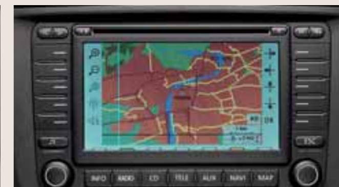
The Nexus navigation system displays the direction of the route, distance to the destination and turning points both on its colour navigation display and within the driver's field of view on the MaxiDOT display. It also allows you to receive traffic reports, play CDs and connect a CD changer.
