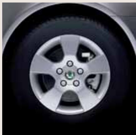
Helios alloy wheels 6.5J x 15" with 205/60 R15 tyres. Standard equipment for the 4x4 Elegance version. Extra equipment for the Classic, Ambiente, Elegance and 4x4 versions.
