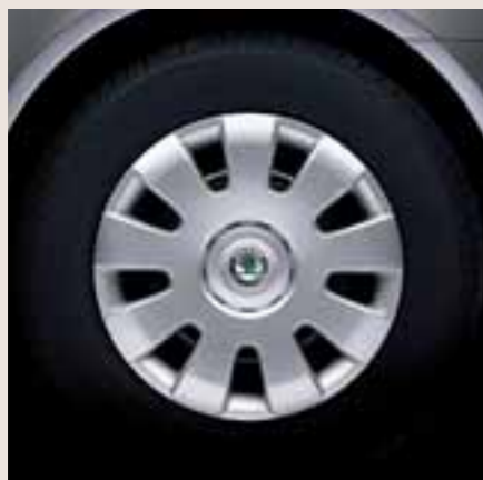
Steel wheels 6.0J x 15" with 195/65 R15 tyres and Castle hub covers. Standard equipment for the Classic version.
