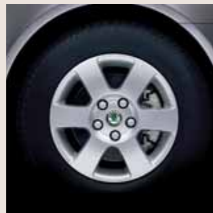
Orion alloy wheels 6.0J x 15" with 195/65 R15 tyres. Standard equipment for the Elegance version.
